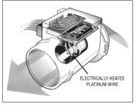
airflow sensor The device in a fuel injection system that measures the flow of air through the intake manifold to determine the amount of fuel to be delivered; also called mass airflow sensor.
