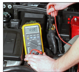
Backprobing ECM connector to check for voltage to LDP solenoid. 13 Engine Management
