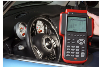
An OBD-II scan tool is invaluable for on-board diagnostics, such as clearing fault codes, and resetting the Check Engine light. OBD On-Board Diagnostics
