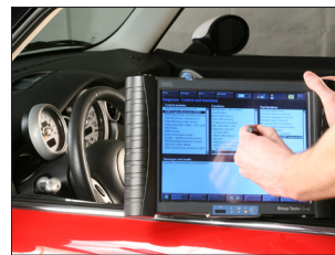
Factory scan tool being used to check power supply (Term. 30) 65 Electronic Immobilization System (EWS)
